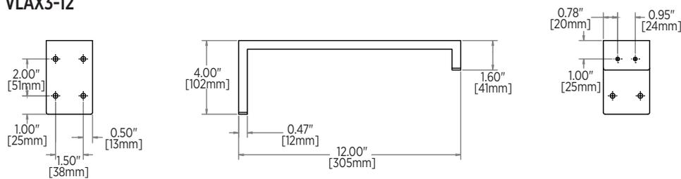
For a standalone installation, use two brackets for each Fixture. If you are installing a continuous run of Fixtures, use one bracket per Fixture, until you reach the last Fixture in the run, where you will install two brackets.
