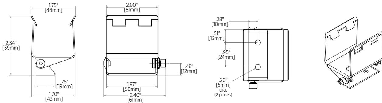
VLA-17 can be adjusted to mount the fixture in a number of different angles.
