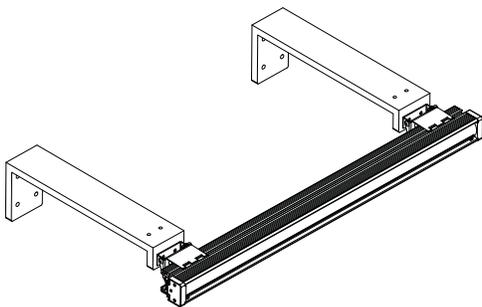
Aluminum mounting arm is designed for extension of the Gen2 Fixture 6 or 12 inches (specify model) from the mounting surface. Extension arm is provided with VLA-17 adjustable mounting bracket.
