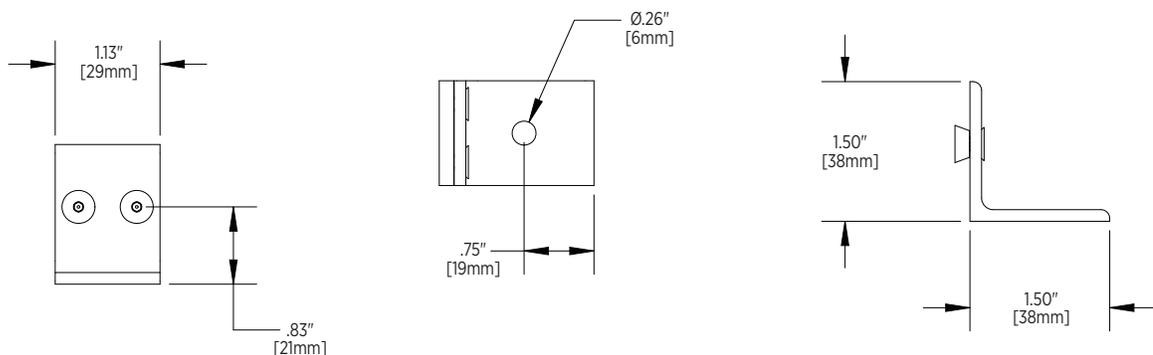
Always use two VLA-9 brackets per Fixture, regardless of whether you are creating a standalone installation or combining any number of Fixtures in a continuous run.
