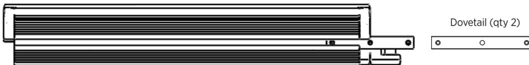
3. Attach second fixture, assuring that the jumper is plugged in correctly and the dovetails are in place.
