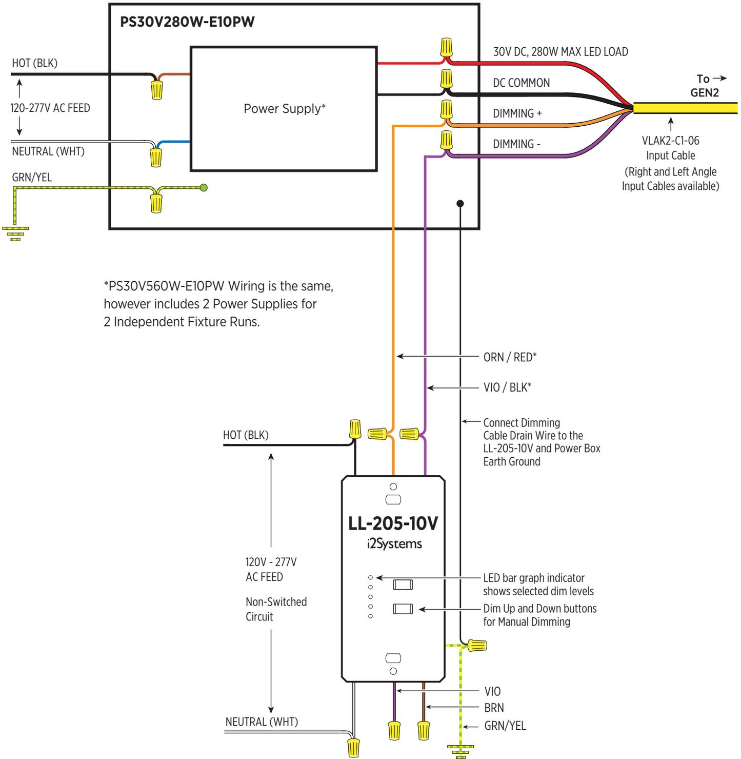
\*Indoor Dimming Cable uses Red and Black Conductors. Outdoor Dimming Cable uses Orange and Violet.
