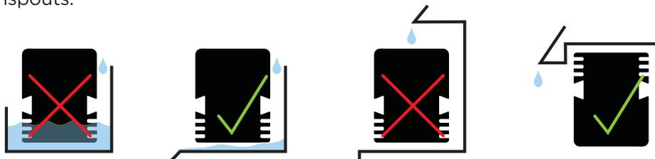
It is good practice to seal all Fixtures and junction boxes with electronics-grade RTV silicone sealant. This will ensure that moisture cannot enter or accumulate in wiring compartments, cables, or other electrical parts when you install the Fixture in wet or damp locations.
